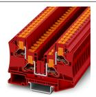
Feed-through terminal block, nom. voltage: 1000 V, nominal current: 41 A, connection method: Push-in connection, Rated cross section: 6 mm², cross section: 0.5 mm² - 10 mm², mounting type: NS 35/7,5, NS 35/15, color: red
