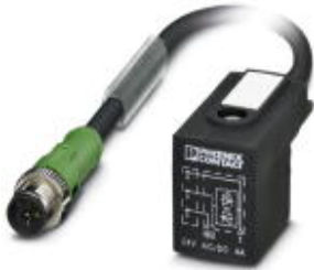
Sensor/Actuator cable, 3-position, PUR halogen-free, Black-gray RAL 7021, Plug straight M12-SPEEDCON, A-coded, on B valve plug (10 mm), with 1 LED, connected with Z diode, Cable length: 0.6 m
