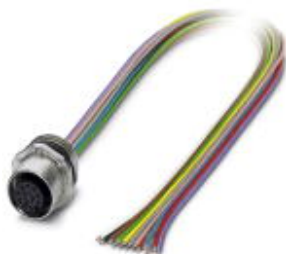
Sensor/actuator flush-type socket, 12-pos., M12 SPEEDCON, front/screw mounting with M16 thread, with 1.0 m PVC litz wire, 12 x 0.14 mm²
