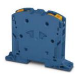
High-current terminal block, Connection method: Power-Turn connection, Cross section: 10 mm<sup>2</sup> - 70 mm<sup>2</sup>, AWG: 8 - 2/0, Width: 20 mm, Color: blue, Mounting type: NS 35/15
