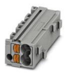
Marshalling patchboard, Nom. voltage: 500 V, Nominal current: 17.5 A, Cross section: 0.14 mm² - 2.5 mm², AWG: 12 - 26, Connection type: Push-in connection, Number of positions: 1, Number of connections: 4, Width: 11 mm, Length: 8.6 mm, Color: gray, Color of connection elements: gray, Assembly: for snapping onto a DIN rail adapter, for snapping onto a cover flange
