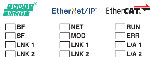
Figure 30 LED status indicators for PROFINET, EtherNet/IP™, EtherCAT®
