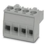
Plug component, Nominal current: 16 A, Rated voltage (III/2): 320 V, Number of positions: 4, Pitch: 5 mm, Connection method: Screw connection
