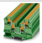
Feed-through terminal block, nom. voltage: 1000 V, nominal current: 41 A, connection method: Push-in connection, Rated cross section: 6 mm², cross section: 0.5 mm² - 10 mm², mounting type: NS 35/7,5, NS 35/15, color: green
