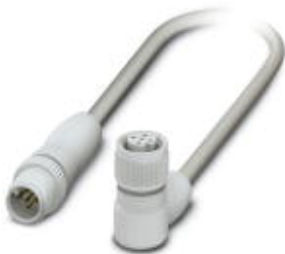
Sensor/Actuator cable, 5-position, PP-EPDM halogen-free, Gray RAL 7035, Plug straight M12, A-coded, on Socket angled M12, A-coded, with 3 LEDs, Cable length: 0.6 m, Hygienic design, with plastic knurl
