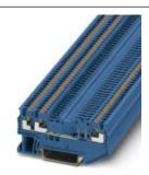
Disconnect terminal block, Connection type: Push-in connection, Cross section: 0.14 mm² - 1.5 mm², AWG: 26 - 14, Nominal current: 10 A, Nominal voltage: 400 V, Length: 67.8 mm, Width: 3.5 mm, Color: blue, Assembly: NS 35/7,5, NS 35/15
