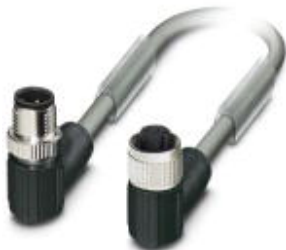
Bus system cable, CANopen®, 5-position, PUR halogen-free, Gray RAL 7001, shielded, Plug angled M12-SPEEDCON, A-coded, on Socket angled M12-SPEEDCON, A-coded, Cable length: 0.5 m
