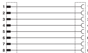
Contact assignment of M12 connector/socket
