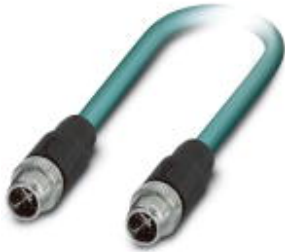
Assembled Ethernet cable, CAT6 A , shielded, 4-pair, AWG 26 stranded (7-wire), RAL 5021 (water blue), M12 connector on M12 connector, length 0.5 m
