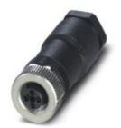
Power connectors, 4-position, Socket straight M12, T-coded, Screw connection, Knurl material: Zinc die-cast, nickel-plated, Cable gland Pg9, External cable diameter 6 mm ... 8 mm, for direct current up to 12 A/60 V
