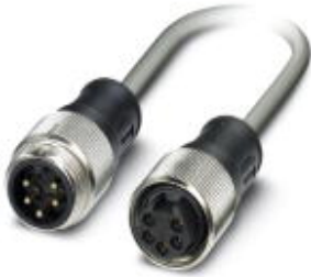
Bus system cable, DeviceNet, 5-position, PUR halogen-free, Gray RAL 7001, Plug straight 7/8"-16UNF, on Socket straight 7/8"-16UNF, Cable length: 0.3 m
