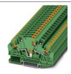
Test disconnect terminal block, nom. voltage: 1000 V, nominal current: 30 A, connection method: Push-in connection, Rated cross section: 6 mm<sup>2</sup>, cross section: 0.5 mm<sup>2</sup> - 6 mm<sup>2</sup>, color: green
