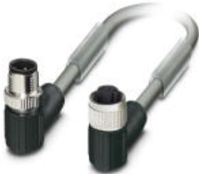
Bus system cable, CANopen®, 5-position, PUR halogen-free, Gray RAL 7001, shielded, Plug angled M12-SPEEDCON, A-coded, on Socket angled M12-SPEEDCON, A-coded, Cable length: 0.3 m
