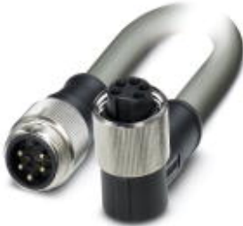
Bus system cable, DeviceNet, 5-position, PVC, Gray RAL 7001, Plug straight 7/8"-16UNF, on Socket angled 7/8"-16UNF, Cable length: 15 m
