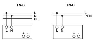
The 100...240 V AC connection is made using the L and N screw connections.
