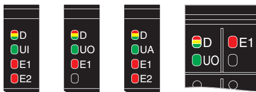
Figure 8-2 LEDs on the power connectors (examples)
