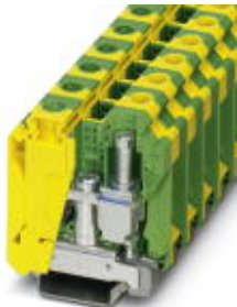
Ground modular terminal block, with screwfix, Connection method: Screw connection, Cross section: 1.5 mm² - 35 mm², AWG: 16 - 2, Width: 16 mm, Color: green-yellow, Mounting type: NS 35/7,5, NS 35/15
