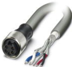
Bus system cable, DeviceNet, 5-position, PVC, Gray RAL 7001, Free cable end, on Socket straight 7/8"-16UNF, Cable length: 15 m
