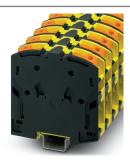
High-current terminal block, nom. voltage: 1000 V, nominal current: 232 A, connection method: Power-Turn connection, 1 level, cross section: 25 mm² - 95 mm², mounting type: NS 35/15, color: black/yellow
