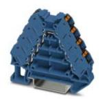
Potential distributors, Nom. voltage: 250 V, Nominal current: 17.5 A, Cross section: 0.14 mm<sup>2</sup> - 2.5 mm<sup>2</sup>, AWG: 14 - 26, Connection type: Push-in connection, Width: 8.3 mm, Length: 64 mm, Color: blue, Assembly: NS 35/7,5, NS 35/15
