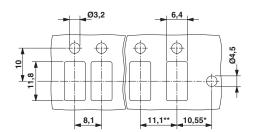
\* Only when using the UW...-F flange plate \*\* Dimensions when using the DP-UW... spacer plate
