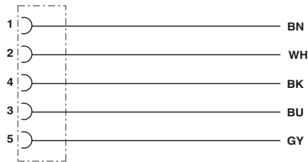
Contact assignment of the M12 socket
