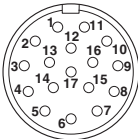
Connector pin assignment M23 socket, 17-pos., female side view
