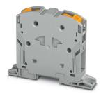
High-current terminal block, nom. voltage: 1000 V, nominal current: 232 A, connection method: Power-Turn connection, 1 level, cross section: 25 mm² - 95 mm², mounting type: direct screw connection, color: gray
