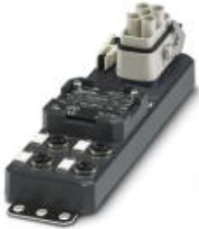
Power distributor, Application: Power supply, Connection method: M12-SPEEDCON-socket Metal, Number of slots: 4, Number of positions: 4, Coding: T power, Slot assignment: single, Status indication: Yes, Universal; Master cable connection: Plug-in master cable connection 90°, Shielding: No
