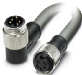
Bus system cable, DeviceNet, 5-position, PVC, Gray RAL 7001, Plug angled 7/8"-16UNF, on Socket straight 7/8"-16UNF, Cable length: 0.5 m
