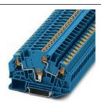
Test disconnect terminal block, nom. voltage: 1000 V, nominal current: 30 A, connection method: Push-in connection, Rated cross section: 6 mm², cross section: 0.5 mm² - 6 mm², color: blue
