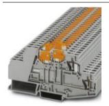
Knife disconnect terminal block, Connection type: Spring-cage connection, Cross section: 0.2 mm² - 4 mm², AWG: 24 - 12, Nominal current: 16 A, Nominal voltage: 400 V, Length: 107 mm, Width: 6.2 mm, Color: blue, Assembly: NS 35/7,5, NS 35/15
