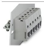
Panel feed-through terminal block, Connection method: Screw connection, Cable lug connection, Load current: 232 A, Cross section: 35 mm² - 95 mm², AWG 4 - 2/0, Connection direction of the conductor to plug-in direction: 0 °, Width: 25 mm, Color: gray
