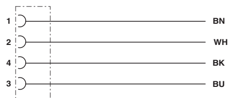
Contact assignment of M8/M12 plugs/sockets
