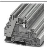
Multi-level terminal block, Connection method: Screw connection, Cross section: 0.14 mm<sup>2</sup> - 6 mm<sup>2</sup>, AWG: 26 - 10, Width: 6.2 mm, Height: 60.1 mm, Color: gray, Mounting type: NS 35/7,5, NS 35/15
