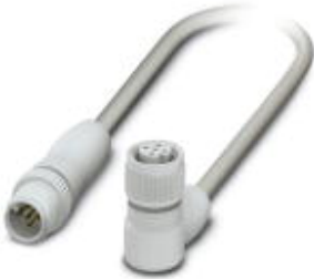
Sensor/Actuator cable, 5-position, PP-EPDM halogen-free, Gray RAL 7035, Plug straight M12, A-coded, on Socket angled M12, A-coded, with 3 LEDs, Cable length: 3 m, Hygienic design, with plastic knurl
