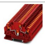
Test disconnect terminal block, nom. voltage: 1000 V, nominal current: 30 A, connection method: Push-in connection, Rated cross section: 6 mm², cross section: 0.5 mm² - 6 mm², color: red
