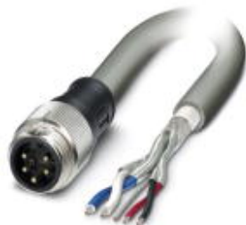
Bus system cable, DeviceNet, 5-position, PVC, Gray RAL 7001, Plug straight 7/8"-16UNF, on Free cable end, Cable length: 15 m
