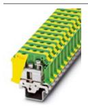
Ground modular terminal block, Screw connection, Cross section: 0.75 mm<sup>2</sup> - 35 mm<sup>2</sup>, AWG: 18 - 2, Width: 15 mm, Color: green-yellow, Mounting type: NS 35/15-2,3, NS 35/15, NS 32
