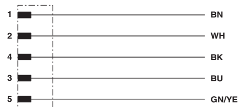
Contact assignment of the M12 plug
