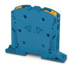
High-current terminal block, nom. voltage: 1000 V, nominal current: 232 A, connection method: Power-Turn connection, 1 level, cross section: 25 mm² - 95 mm², mounting type: direct screw connection, color: blue
