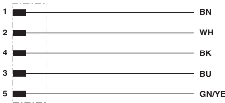
Contact assignment of the M12 plug
