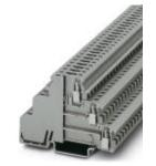
Sensor/actuator terminal block, with integrated diode, Cross section: 0.2 mm<sup>2</sup> - 4 mm<sup>2</sup>, AWG: 24 - 12, Connection type: Screw connection, Width: 6.2 mm, Color: gray, Mounting type: NS 35/7,5, NS 35/15
