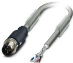
Bus system cable, CANopen®, 5-position, PUR halogen-free, Gray RAL 7001, shielded, Plug straight M12-SPEEDCON, A-coded, on Free cable end, Cable length: 5 m
