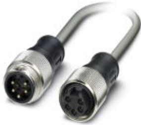
Bus system cable, DeviceNet, 5-position, PUR halogen-free, Gray RAL 7001, Plug straight 7/8"-16UNF, on Socket straight 7/8"-16UNF, Cable length: 1 m
