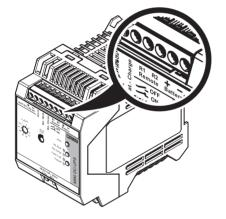
The rechargeable battery module is connected to the power supply unit through the "Battery +" and the "Battery -" terminal blocks. The fuse of the rechargeable battery module must be removed when installing or replacing the module.
