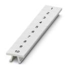
Zack marker strip, Strip, white, labeled, can be labeled with: CMS-P1-PLOTTER, Printed vertically: consecutive numbers 1  $\dots$  10, 11  $\dots$  20, etc. up to 491  $\dots$  500, mounting type: snap into tall marker groove, for terminal block width: 6.2 mm, lettering field size: 6.15 x 10.5 mm, Number of individual labels: 10
