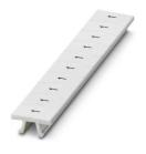
Zack marker strip, Strip, white, labeled, can be labeled with: CMS-P1-PLOTTER, printed horizontally: Identical numbers 1 or 2, etc. up to 100, mounting type: snap into tall marker groove, for terminal block width: 6.2 mm, lettering field size: 6.15 x 10.5 mm, Number of individual labels: 10
