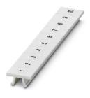
Zack marker strip, Strip, white, labeled, can be labeled with: CMS-P1-PLOTTER, printed horizontally: consecutive numbers 1 ... 10, 11 ... 20, etc. up to 491 ... 500, mounting type: snap into tall marker groove, for terminal block width: 6.2 mm, lettering field size:  $6.15 \times 10.5 \text{ mm}$ , Number of individual labels: 10
