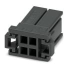
PCB connector, color: black, nominal current: 8 A, rated voltage (III/2): 160 V, contact connection type: Socket, number of rows: 2, number of positions: 4, product range: DD31PC 2,2/..., pitch: 3.81 mm, connection method: Crimp connection, conductor/PCB connection direction: 0 °, locking clip: - without locking clip, plug-in system: CONNEXIS DD, locking: Snap-in locking, mounting: Self-locking flange, type of packaging: packed in cardboard
