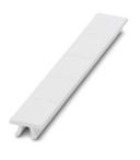
Zack marker strip, Strip, white, unlabeled, can be labeled with: PLOTMARK, CMS-P1-PLOTTER, mounting type: snap in, for terminal block width: 16 mm, lettering field size: 16 x 10.5 mm, Number of individual labels: 50
