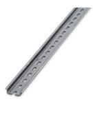
DIN rail perforated, acc. to EN 60715, material: Steel, Galvanized, white passivated, Standard profile, color: silver, Pack of 25 (50 m)
