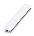
Marker for terminal blocks, Strip, white, labeled, can be labeled with: CMS-P1-PLOTTER, printed horizontally: U, V, W, N, GND, U, V, W, N, GND, mounting type: snap into tall marker groove, for terminal block width: 6.2 mm, lettering field size: 6.15 x 10.5 mm, Number of individual labels: 10
