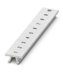
Zack marker strip, Strip, white, labeled, can be labeled with: CMS-P1-PLOTTER, printed horizontally: consecutive numbers 1 ... 10, 11 ... 20, etc. up to 491 ... 500, mounting type: snap into tall marker groove, for terminal block width: 6.2 mm, lettering field size:  $6.15 \times 10.5$  mm, Number of individual labels: 10
